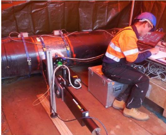
**Figure 3** LDV Installation for In situ Calibrations (Johnson, et al , 2016)
