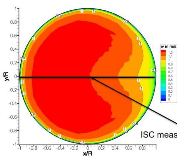
**Figure 2** Velocity profile distortion due to an upstream 15° bend (source : Optolution)
