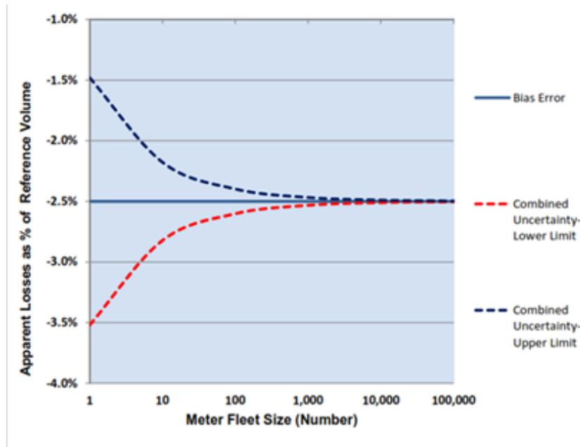
Figure 1 Combined meter measurement errors (Johnson, 2012)
